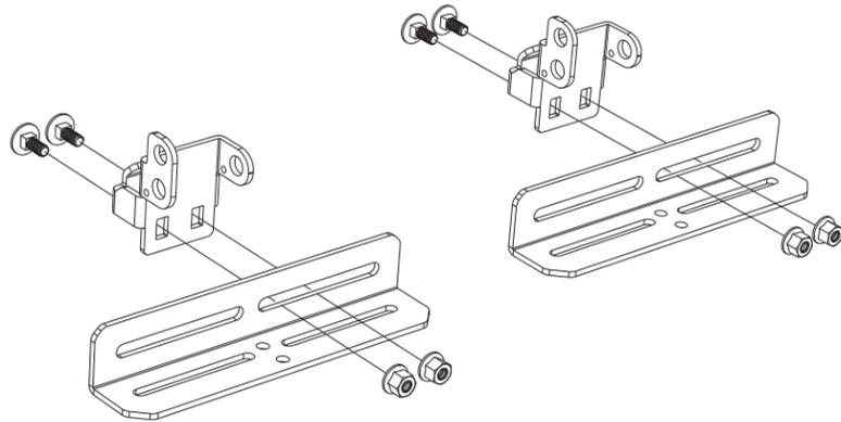
ASSEMBLE TWO PINNED BRACKET ASSEMBLIES AS SHOWN, USING M6 CARRIAGE BOLTS AND LOCKNUTS. ONLY PARTIALLY TIGHTEN NUTS TO ALLOW FINAL ADJUSTMENT WITH CASE POSITION.
