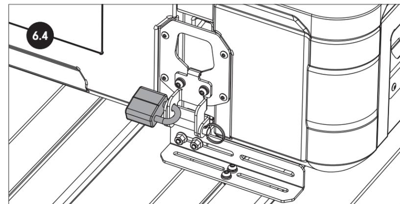
1. SQUEEZE END OF LANYARD AND PUSH THROUGH HOLE IN PINNED YOKE
