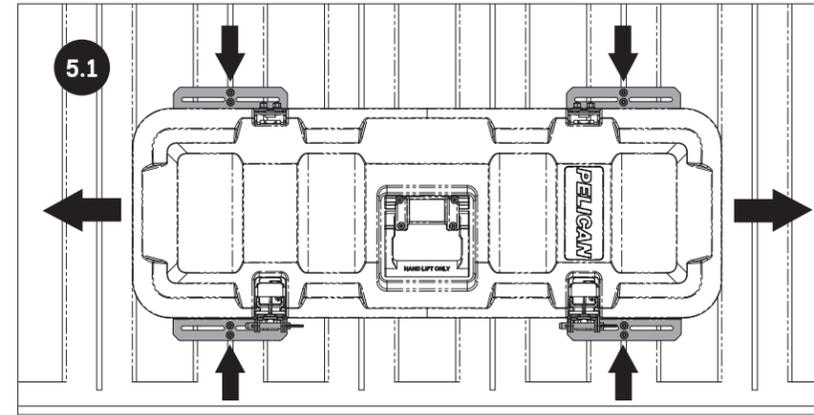
PLACE CARGO CASE IN DESIRED POSITION ON YOUR ROOF RACK.
