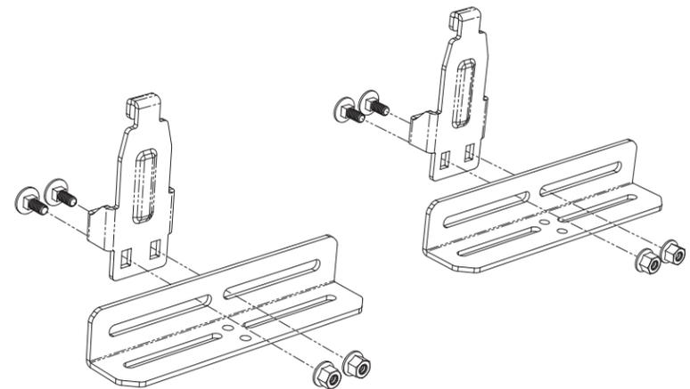
ASSEMBLE TWO FIXED BRACKET ASSEMBLIES AS SHOWN, USING M6 CARRIAGE BOLTS AND LOCKNUTS. ONLY PARTIALLY TIGHTEN NUTS TO ALLOW FINAL ADJUSTMENT WITH CASE POSITION.
