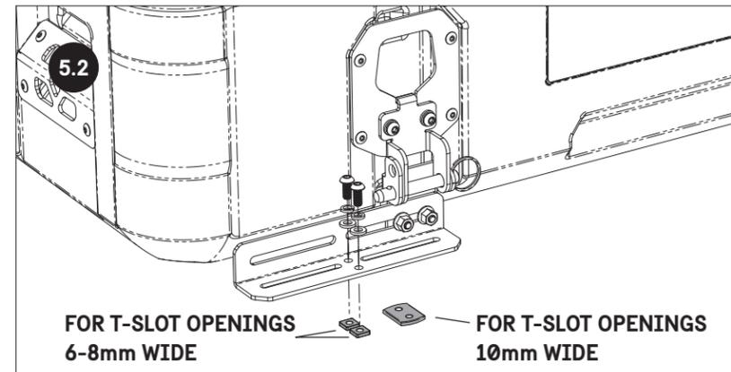
INSERT M6 SCREWS WITH FLAT AND LOCK WASHERS INTO THE 4 MOUNTING BRACKETS.
