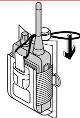
Click the release buckle together, then pull the bungee cord tight while sliding the cord lock towards the holster.
