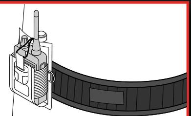
Attach to a tool belt or harness using either the velcro strap or sewn loop on the back of the holster.
