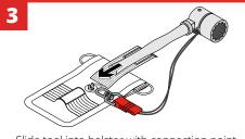
Slide tool into holster with connection point applied to tool.
