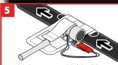
Apply holster to your work belt, by sliding belt through the slip located on the upper end of holster.
