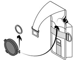
Remove tool ring from Retractor then insert Retractor into holster pocket. Feed end of Retractor cable out of holster pocket.
