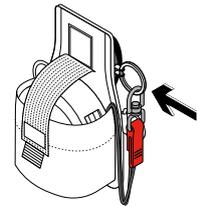
Tether your tool or GRIPPS® Swivel Catch directly to the retractor unit tool ring.
