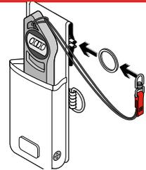
Thread tool ring back onto Retractor. The tool ring should be exposed outside of the holster.
