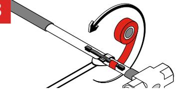
Apply GRIPPS® V-Gripp Tape to the straps/wings of the Tool Hitch. Wrap around 10x times on either side.
