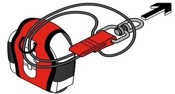
If using a GRIPPS® Swivel Catch, feed cord through D-Ring on the back of Tape Measure Catch. Then attach to the tooling from the retractor unit.
