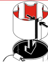
Open tool bag and insert Lifting Bag Insert in main compartment, bending as required. Ensure velcro edges are joined evenly and overlaps.
