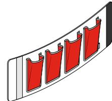
Lay out Lifting Bag insert and begin to flex into a circular shape, keeping pockets on the inside of the ring created.
