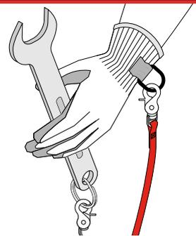
Once the tool ring is applied to your chosen tool, connect the tool ring to a GRIPPS® tether of choice.
