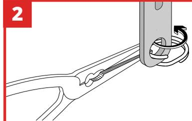
Using the needle nose pliers, thread the pried-open halves of the Tool Ring into the tool aperture. Rotate the Tool Ring until both halves of the Tool Ring are inside the tool aperture and the tool is secured.
