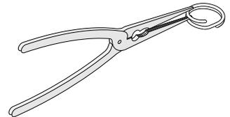
Pry the two halves of Tool Ring open with a set of ring pliers or needle nose pliers.
