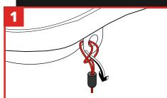
Feed the looped end of the hard hat tether through an appropriate connector point on the hard hat.
