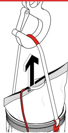
Only lift from the clearly identified load-rated lifting point on the straps, and ensure tools are tethered to the D-Rings at all times. Do not lift from carabiner.
