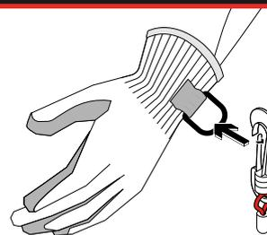
Open/Close Carabiner as required. Push carabiner into anchor point or tool connection point.
