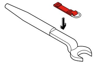
Place Tool Catch with metal ring facing away from the tools center of gravity, white tag facing up.
