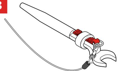
Your Tool Catch is now ready to be connected with a suitable GRIPPS® tether via the D-Ring.
