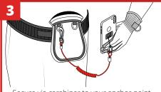
Secure via carabiner to your anchor point. Press side-release buttons to hot-swap between different electronic devices. Ensure attachment dock 'clicks' back into place.
