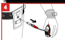
Attach holster to your work belt by sliding belt through the rear straps of the Tape Measure Latch Holster.
