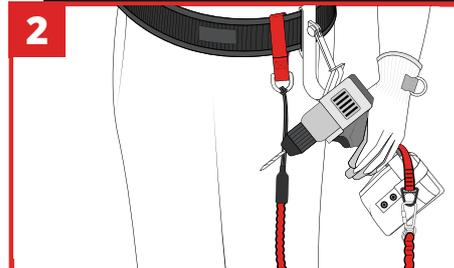
Your tethered drill (or similar device) can be stowed into the BOA after by simply pressing your tool into the latch. The latch utilizes a spring to automatically lock after. To remove your tool, press latch inwards and pull tool out. Ensure your tool is properly anchored before using BOA holster.
