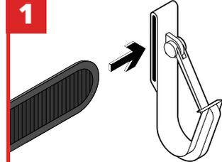
To connect to a work belt, thread work belt through the loop of Battery Operated Arrest Holster.
