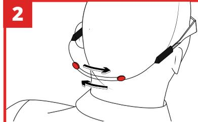
Place eyewear and Safety Glasses Tether on head. Adjust the Safety Glasses Tether by sliding the two red central pieces to opposite sides.
