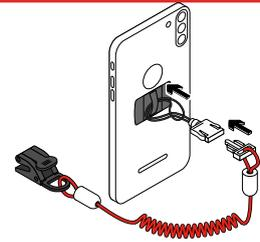
Secure E-Tether to E-Catch by first feeding loop through the connector point, then feed the E-Tether back through the loop to create a choke.
