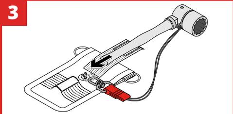
Slide tool into holster with connection point applied to tool.
