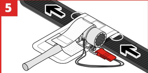
Apply holster to your work belt, by sliding belt through the slip located on the upper end of holster.
