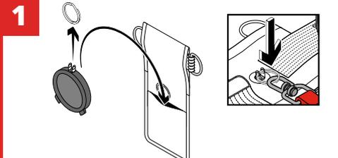
Remove tool ring from Retractor unit then insert into back pouch of holster. Reattach tool ring, keeping the ring exposed outside holster.
