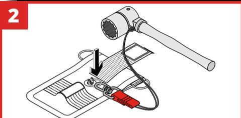
Connect tool to the Retractor or side D-Rings.
