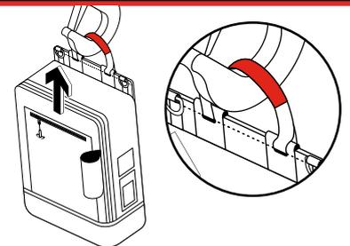
Ensure all tools are tethered to D-Rings and zips fully sealed. Attach lifting hook to the red upper lifting strap.
