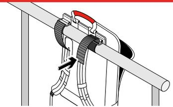
To secure to a rail, wrap the straps all the way around the rail and feed back through the metal bracket.
