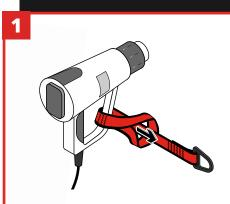
Pass one end of the Tool Hitch around the neck (near the tool's center of gravity). Then pass the D-Ring end back through the Tool Hitch loop to create a choke-hold.
