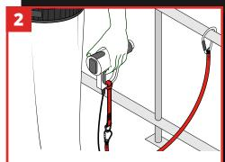
Your Tool Hitch is now ready to be tethered to a suitable anchor point using an appropriate GRIPPS® Tool Tether.
