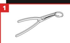
Pry the two halves of Tool Ring open with a set of ring pliers or needle nose pliers.
