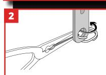
Using the needle nose pliers, thread the pried-open halves of the Tool Ring into the tool aperture. Rotate the Tool Ring until both halves of the Tool Ring are inside the tool aperture and the tool is secured.
