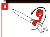
Wrap the tape around the tool 10x while stretching the tape to activate the self-vulcanizing feature, creating a secure connection. Ensure raised 'catch' is not covered by the tape. Pull on Tool Catch with force to test application.
