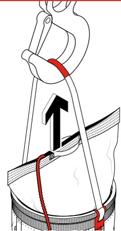
Only lift from the clearly identified load-rated lifting point on the strap, and ensure tools are tethered to the D-Rings at all times. Do not lift from carabiner.
