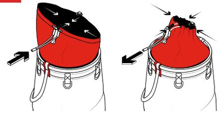
To secure contents inside the Scaffold Tube Lifting Bag, pull the drawstring tight.
