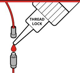
Squeeze a drop of thread-locking compound onto thread for a permanent connection point.
