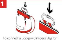
To connect a Lockjaw Climbers Bag for personal use, feed a carabiner through either the upper or lower set of loops.
