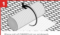
Place roll of GRIPPGrid on gridmesh floor in desired location. Roll out matting ensuring material is flat without kinks.
