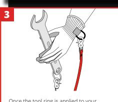
Once the tool ring is applied to your chosen tool, connect the tool ring to a GRIPPS® tether of choice.
