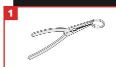
Pry the two halves of Tool Ring open with a set of ring pliers or needle nose pliers.
