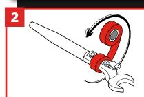
Wrap the tape around the tool 10x while stretching the tape to activate the self-vulcanizing feature, creating a secure connection. Ensure raised 'catch' is not covered by the tape. Pull on Tool Catch with force to test application.
