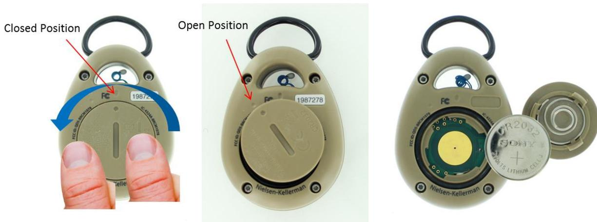
Figure 2: Battery Replacement
