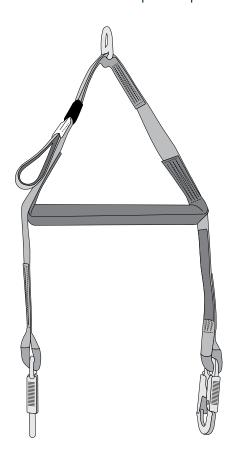
The SpanSet 4006 spreader bar is for use in tight confined space entry applications in line with AS2865 — Safe Working In a Confined Space. It enables a worker to be lifted or lowered while maintaining a straight vertical profile which is not available with a rear D connection. This allows the worker to manoeuvre through tight manholes etc.
