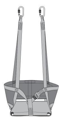
The SpanSet Bosun's chair is a work positioning device only and is not a fall arrest device. It is used in tandem with the 4006 Spreader Bar for short term suspension only. Commonly used with a personnel winch or pulley system. Operators using this equipment must be wearing a full body fall arrest harness (e.g. 1100 ERGO or similar) and be connected to an independent anchorage line via an energy absorber or lanyard (e.g. 3109 Fall Arrest Anchorage Line, 3051 Energy Absorber).
